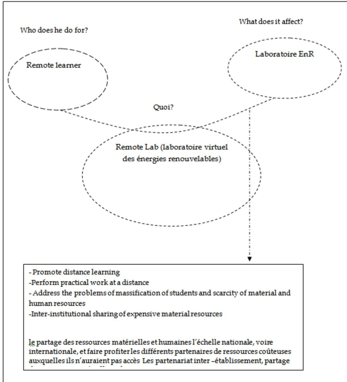
Figure 1 - Functional specifications: "horned beast" diagram
