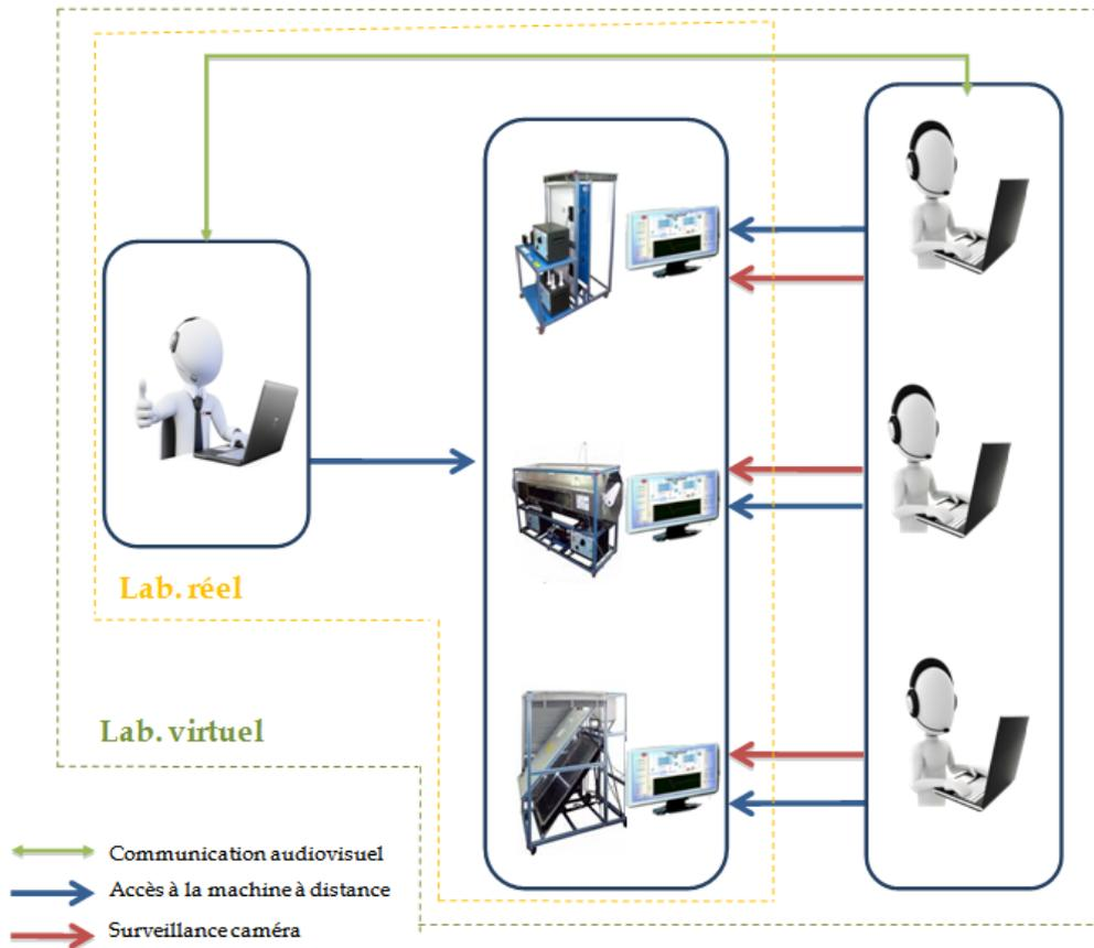
Figure 6 - Architecture du Lab-Vi-EnR
